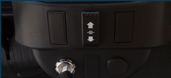
Single Combination Switch for LED Projector Hi & Lo Beam Headlights, LED Signal Lights, Taillights and Horn
