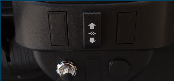
Single Combination Switch for LED Projector Hi & Lo Beam Headlights, LED Signal Lights, Taillights and Horn
